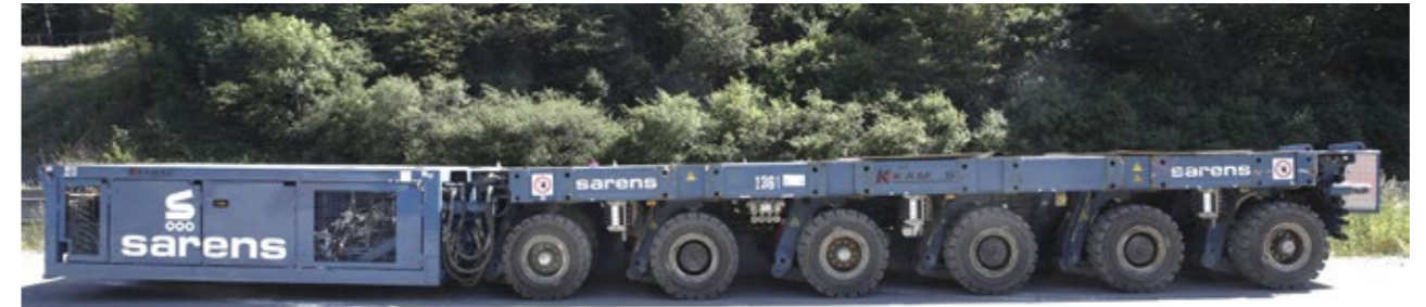
16 such self-propelled platform module transporters (SPMT) of the Ulm manufacturer Kamag transport technology were used for positioning the bridges.
